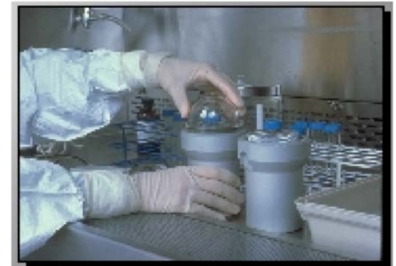
Containment of centrifugation-produced aerosols (use of closed tubes / rotors, opened in BSC)
