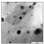
Transmission electron micrograph of rutile TiO<sub>2</sub> nanorod (grey) loaded with Ru nanoparticles (brighter) for the methanation of CO<sub>2</sub>
